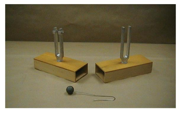
Apparatus: Two tuning forks on wood bases Rubber striker
