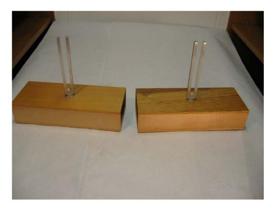
Apparatus: Two tuning forks on wood bases
