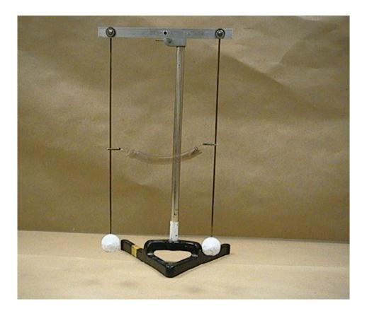
*Apparatus*: Coupled oscillator apparatus
