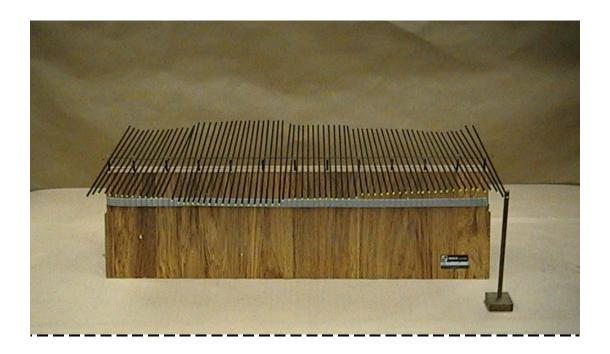
**Apparatus:** Wave demonstrator Termination clamp
