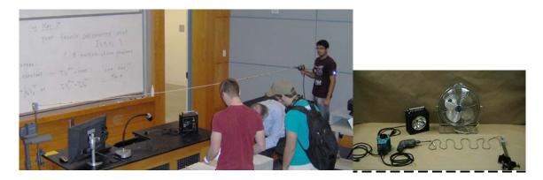
Apparatus: Drill with offset rod and rope attached
