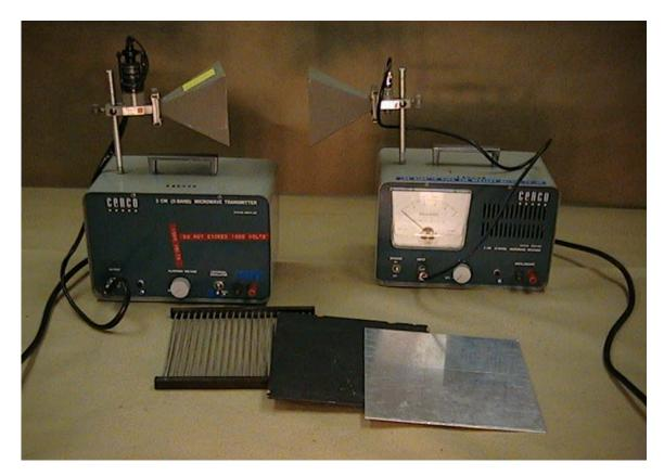
Apparatus: Microwave transmitter and receiver assembly Metal grid plate Aluminum plate Wood-fiber plate
