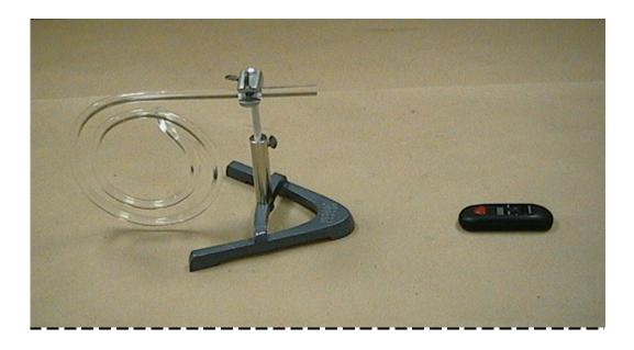
*Apparatus:* Clear curved lucite rod on stand Laser pointer
