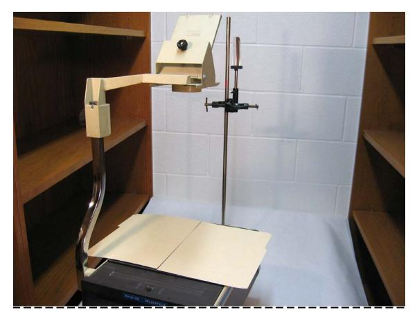
*Apparatus:* Prism on a mount Overhead projector with two card board sheets
