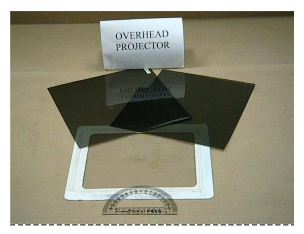
Apparatus: Polaroid sheets (2) Plastic protractor Transparency sheet with "magic" tape Overhead projector
