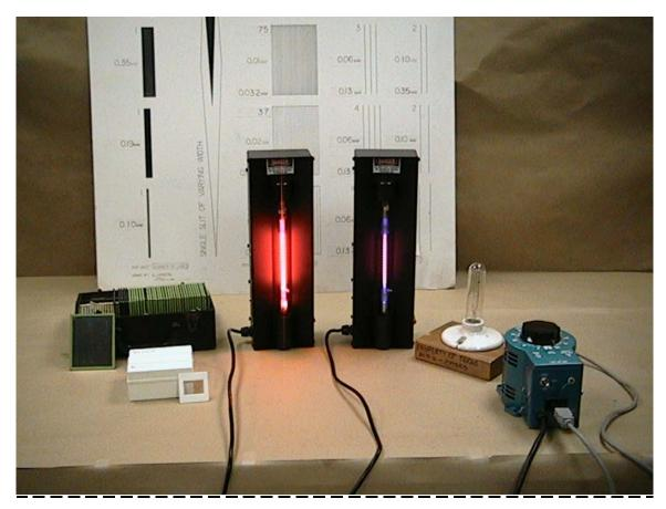
Apparatus:Gas discharge tubes and supports (2 ea)Incandescent lamp on baseDiffraction gratings (specify number)Cornell slides (specify number)Cornell slide pattern board
