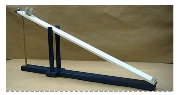
Apparatus: Hinged board apparatus Steel ball Support stick
