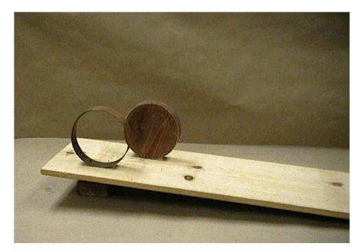
Apparatus: Wood board (1ft x 3ft) Spacers (2 wood blocks) Solid wood disk Thin metal ring
