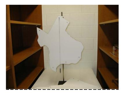
Apparatus:White boards (assortment)<br/>Long rod and base with a two-way clamp<br/>String and plumb bob<br/>Mounting rod (to hold boards and plumb bob)
