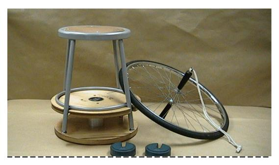
*Apparatus:* Bike wheel with rope attached Rotating platform and attached chair 2Kg masses (2)
