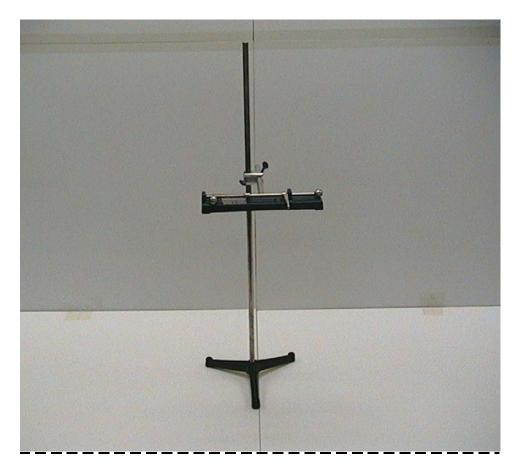
*Apparatus:* Drop and shoot apparatus w/ two steel balls Two-way clamp, rod and base
