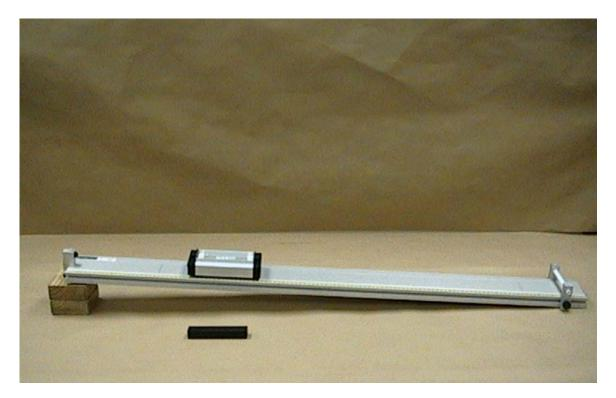
Apparatus:Pasco Linear Track<br/>Pasco cart<br/>1 black metal block<br/>Wood spacers (2 ea, to elevate the track)
