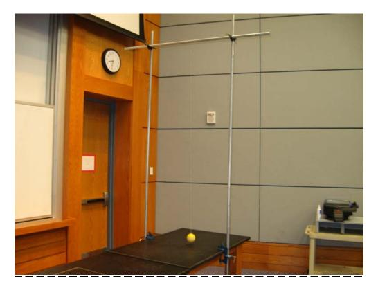
*Apparatus:* Wood ball with string attached 2 long (8ft) rods, 2 table clamps, 2 two-way clamps and a long cross member rod
