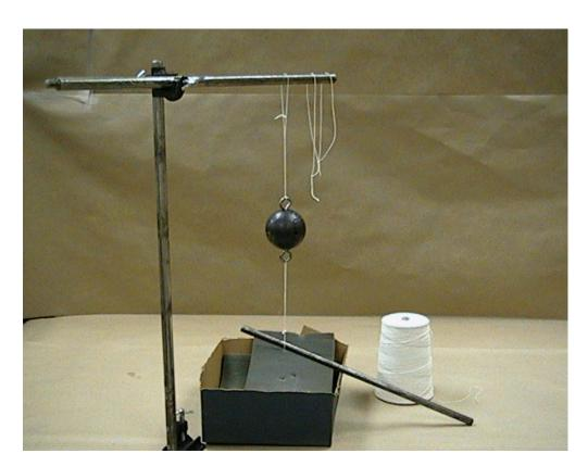
Apparatus: A frame consisting of a table clamp with a long <sup>3</sup>/<sub>4</sub> inch OD steel rod attached vertically and a two-way clamp with a short steel rod extending to one side. Steel ball (about 8 cm diameter, with 2 eyehooks) Cardboard box with foam inside (to catch steel ball) Short steel rod Ball of light-weight string
