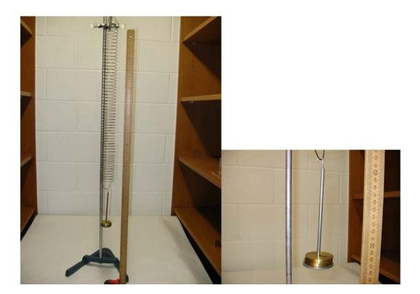
*Apparatus:* Large spring on tall rod and stand Mass hanger 2 – 50g slotted masses Meter stick and support
