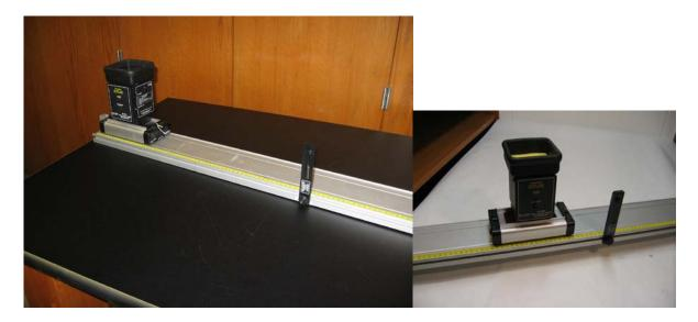
*Apparatus:* Pasco Track Cart/launcher and plastic ball Beam interrupter
