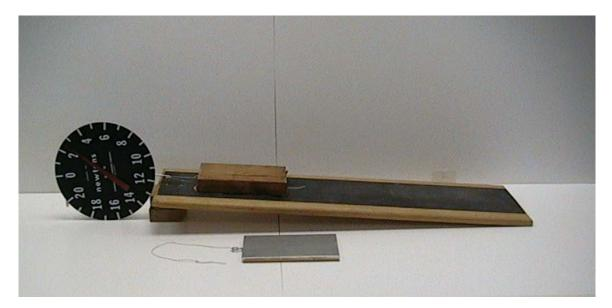
Apparatus:Wood board (1ft x 3ft, with sandpaper strip on one side)<br/>20N spring scale<br/>Wood block (w/string attached)<br/>Aluminum block (w/string attached)<br/>Wood spacers (used to elevate board)
