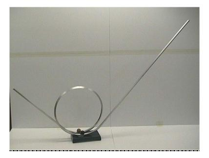
*Apparatus:* Loop the loop apparatus with two balls
