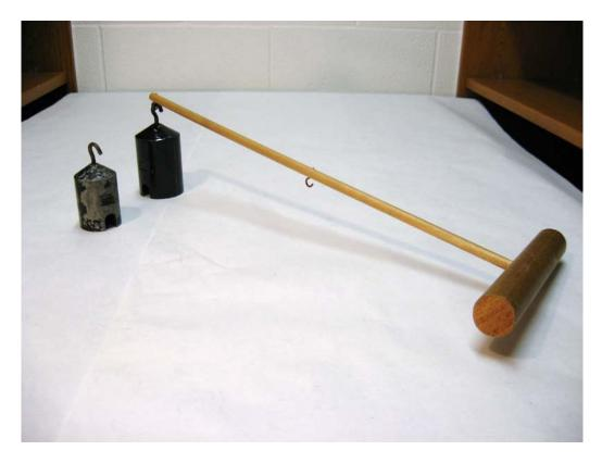
*Apparatus:* Torque rod with hooked masses
