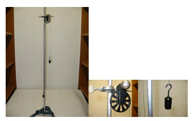
Apparatus:Rod and standTwo way clamp and short rod with steel ballLow friction pulley and string2ea 20 gram hooked masses and a small clip
