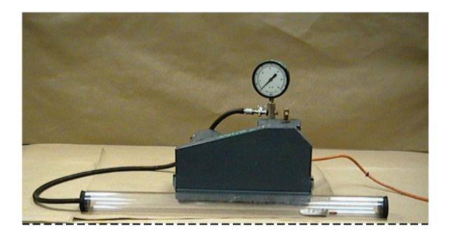
*Apparatus:* Vacuum pump and hose Lucite tube Feather and plastic device (coin substitute)
