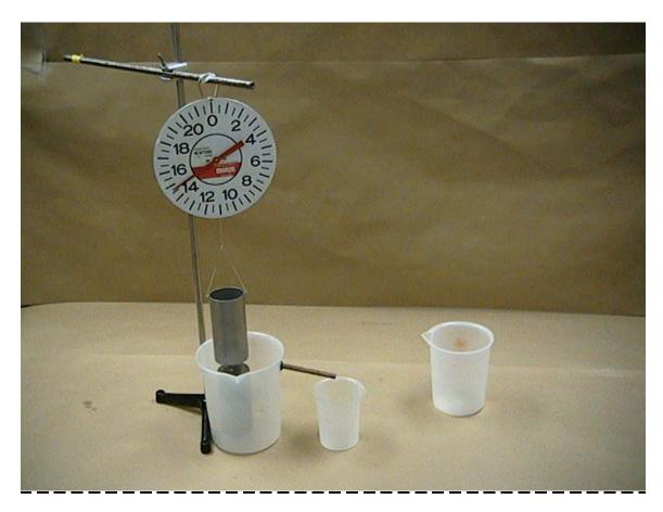
Apparatus:20N spring scale, short rod and two-way clamp<br/>Long rod and base<br/>Metal can with string attached<br/>Cylindrical metal block<br/>Large plastic beaker (with overflow pipe)<br/>Plastic beaker (to catch overflow water)<br/>Small plastic beaker (to help refill large beaker)
