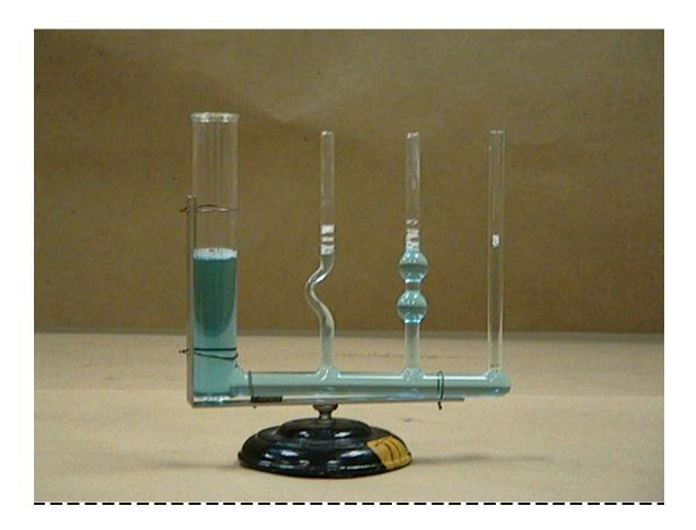
*Apparatus:* Constant level tubes with colored water
