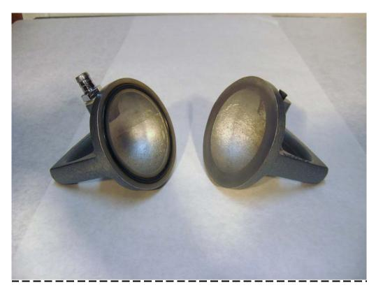
*Apparatus:* Vacuum pump and the hemispheres
