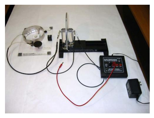
Apparatus: Electroscope (project-o-scope)
