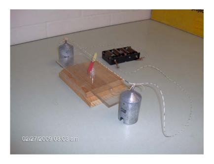
Apparatus: Compass needle on plastic base
