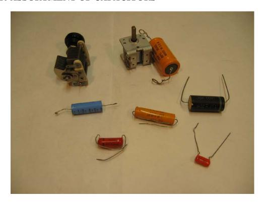
Apparatus: Assortment of capacitors (mica, air, variable, electrolytic)
