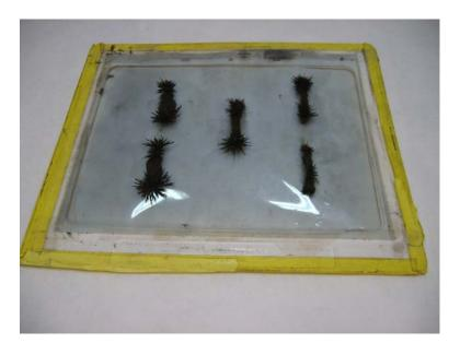
Apparatus: Clear plastic sheet with magnets glued to the inside.
