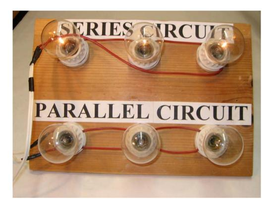
Apparatus: Circuit board with light bulbs in series and parallel
