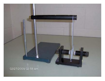
Apparatus: Eddy current apparatus and set of attachments
