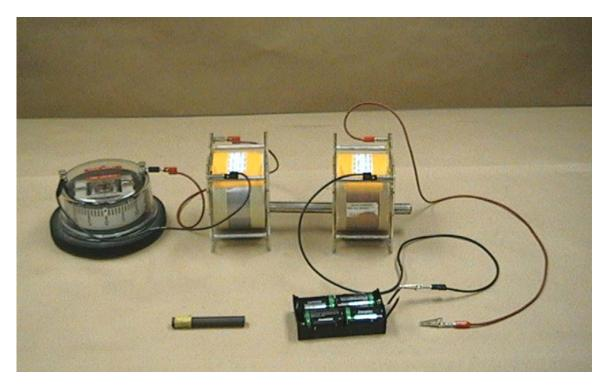
Apparatus: Galvanometer 2 Large coils
