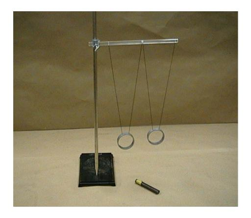
Apparatus: 2 metal rings on a lucite rod attached to a rod and base
